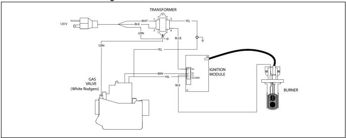
If any of the original wire as supplied with the heater must be replaced, it must be replaced with wiring material having a temperature rating of at least 105°C and 600 volts.
