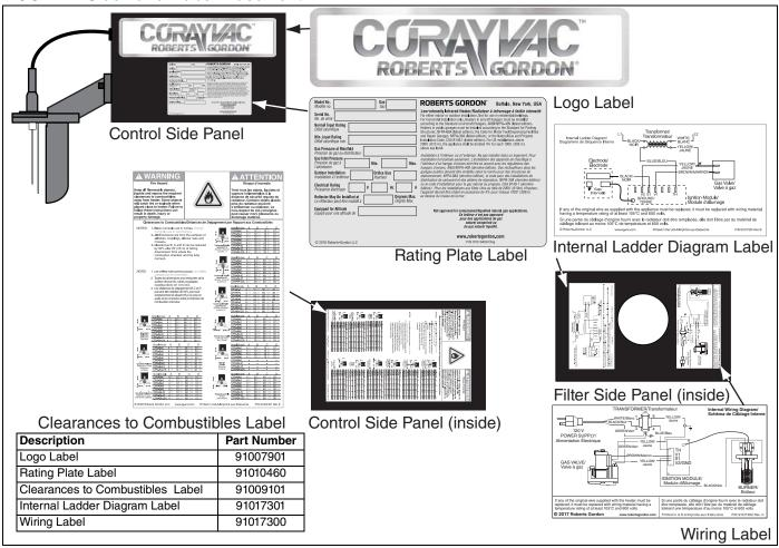
FIGURE 2: Top and Back Panel Label Placement
